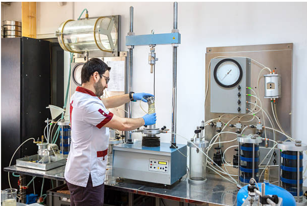
Geotechnical engineer setting up triaxial test on soil sample
